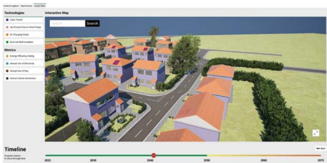
Figure 7: Street view in the year 2041. Solar panels are highlighted in purple, as the user has selected those in the sidebar. Other low carbon technologies are also shown: external wall insulation is indicated by light purple colouring of houses, and an EV charging point is visible as a short post next to the driveway of one house. Heat pumps are also shown in this view, but none are visible in this screenshot.
