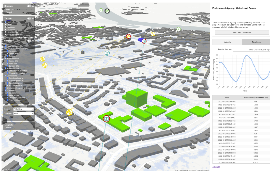
Figure 20: Integration of building and sensor data in the digital twin. Contains OS data. © Crown copyright and database rights 2022.
